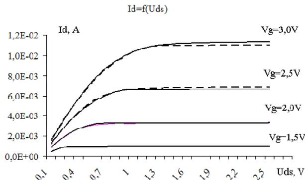
**Figure 2.** Dependence  $I_d=f(D)$  (— experimental, --- simulated) for nonirradiated TMOS.
