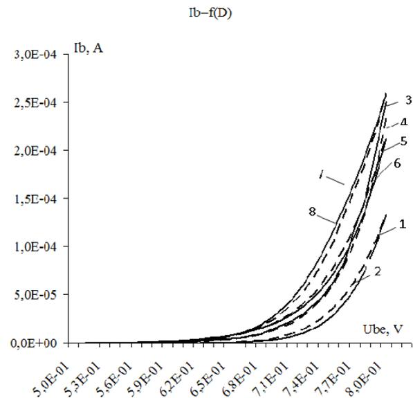
**Figure 1.** Dependence  $I_b=f(U_{be})$  (\_\_\_ experimental, --- simulated) for bipolar transistor: 1, 2 - before irradiation; 3, 4 - irradiated with neutrons,  $D=2.4E+12$  ncm<sup>-2</sup>; 5, 6 - irradiated with  $\gamma$  quanta,  $D=1.2E+5$  Gr(SiO<sub>2</sub>); 7, 8 - irradiated with X-rays,  $D=4.2E+4$  Gr(SiO<sub>2</sub>).
