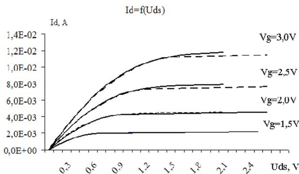
**Figure 3.** Dependence  $I_d=f(U_{ds})$  (— experimental, --- simulated) for TMOS,  $D=3E+4$  Gr(SiO<sub>2</sub>).
